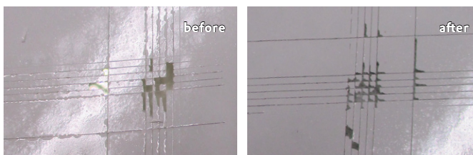
Samples treated with VPS 1178 (cutted before and after 120 min in boiling water)
