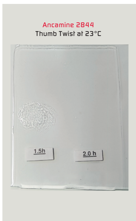
Figure 3: Thumb twist test after 1.5 h and 2 h respectively.
