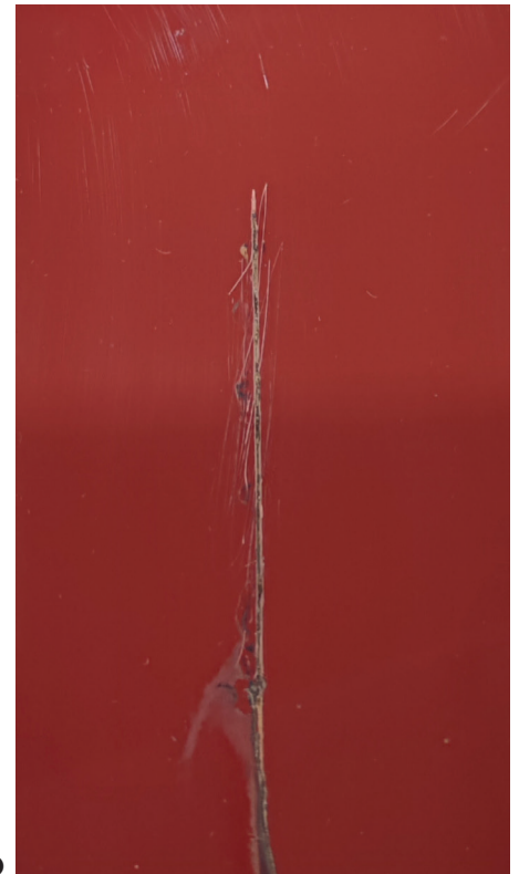
Figure 5: Salt spray test panel after 3000 h.
