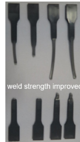
r-HDPE specimen with 2% TEGO® Cycle CP 310
