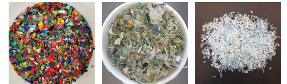
r-HDPE or r-PP Flakes contain 5–10% water without DW 210
