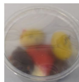
PET-film, 36µm, 5.0 g/m 2 coated with standard heat seal lacquer
