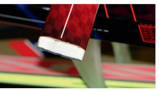
Solid, rigid, and extraordinarily light, ROHACELL\* is an ideal material for lightweight, yet durable skis. Made with a sandwich composite, the skis feature optimal flexibility and dynamics at low weight. Evonik's product is used as a material in box construction—an interior foam core surrounded by a layer of fiberglass-reinforced plastic.
