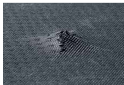
Figure 8: CFRC after 60 J impact. Standard DGEBA epoxy versus ALBIPOX® F 081
