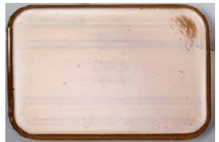
Figure 10: Cured UPES resin without additive and with 0.2 % TEGOMER® D 2345
