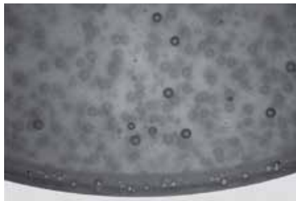
Figure 9: Cured epoxy resin without additive and with 0.3 % TEGOMER® DA 626
