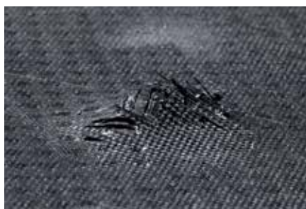
Figure 8: CFRC after 60 J impact. Standard DGEBA epoxy versus ALBIPOX® F 081
