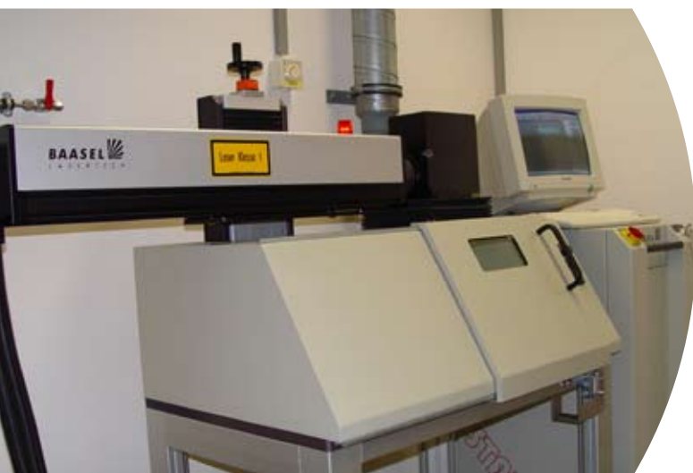
Fig. 13: Nd:YAG marking laser 1064 nm (from Baasel-Lasertechnik)
