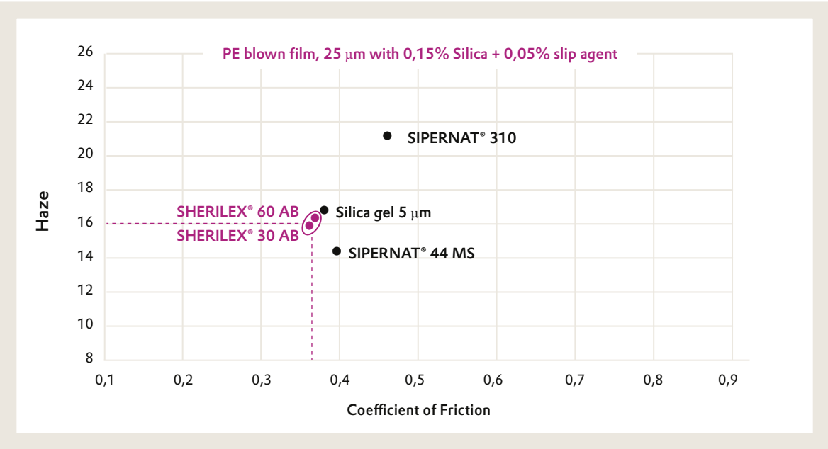
FIGURE 9: SPHERILEX® 30 AB and SPHERILEX® 60 AB provide excellent balance of low Haze and low CoF in PE blown film containing additionally slip agent
