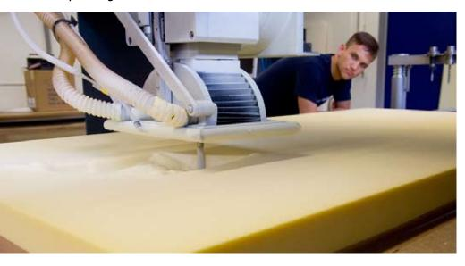
It's up and away from Darmstadt! ROHACELL® is a material that can be perfectly shaped into the cores of sandwich components—as are used in helicopter rotor blades, for example—by using high-precision CNC technology.
