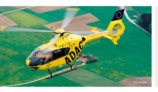
It's all about technology you can trust. The pilot can devote his attention to stabilizing the helicopter and doesn't have to think twice about the rotor blades, the most important component of this aircraft, thanks to their stable sandwich construction—made possible by ROHACELL® rigid foam cores.
