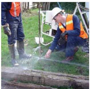
Figure 2 | Low pressure water test of pressure activated tip with 4 horizontal openings
