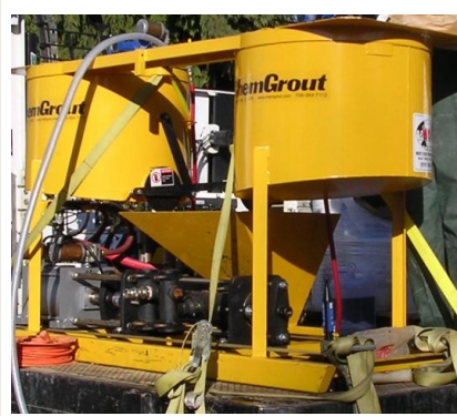
Figure 1 | ChemGrout’s CG-500 mixing unit with high pressure piston pump
