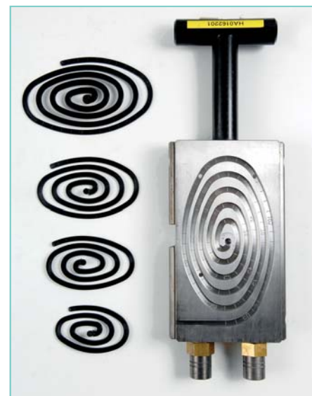
Fig. 6: Spiral tool for the measurement of melt flow index (MFI)
