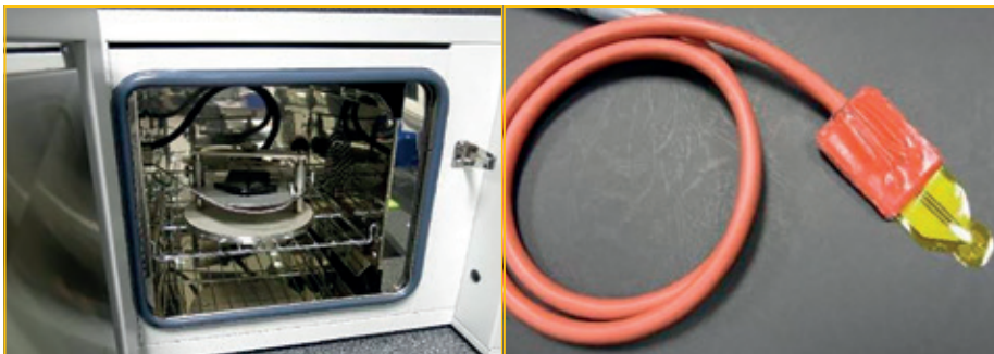
Fig. 3: Material holder and sensor for the hot disk method (heat conductivity measurement)
