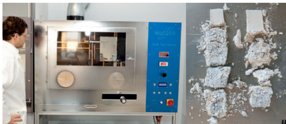
Fig. 9: Flame retardancy test and burned HCR
