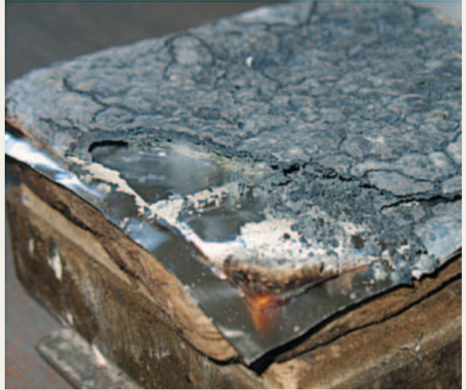
With 2% TEGOMER® V-Si 4042 used during compounding, LOI = 43
