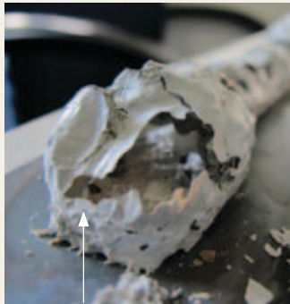
Without additive 2% TEGOMER®V-Si 4042 used during compounding
