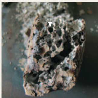
Without additive 2% TEGOMER®V-Si 4042 used during compounding
