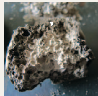
Without additive 2% TEGOMER®V-Si 4042 used during compounding
