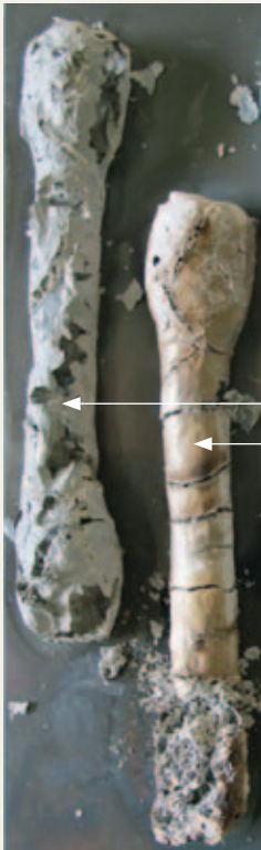
Without additive 2% TEGOMER®V-Si 4042 used during compounding
