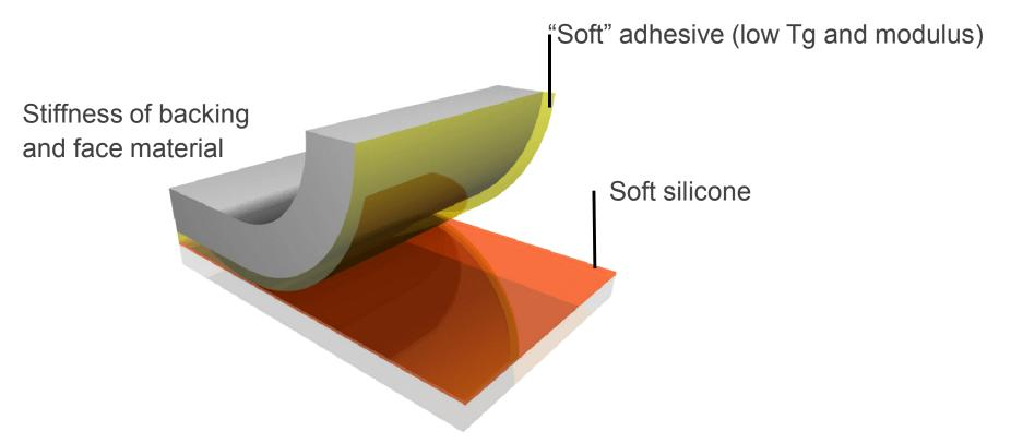
Release is influenced by the test set up and label construction, this is often disregarded as a contributor to release force
