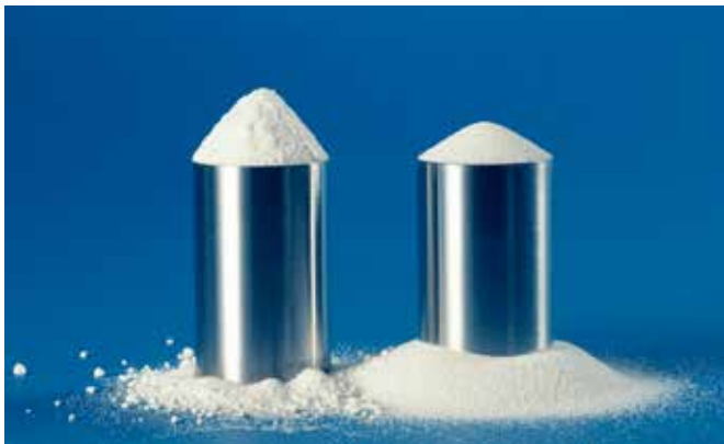
Figure 4 Measuring the angle of repose or cone height on a steel cylinder
