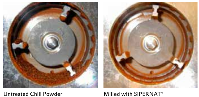
Figure 2 Example of Chili Powder in a hammer mill untreated (left) and treated (right) with SIPERNAT® precipitated silica
