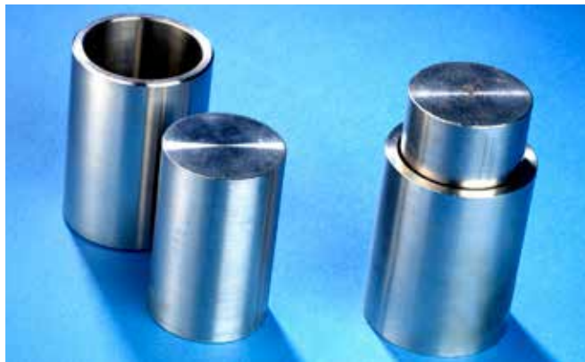
Figure 6 Steel cylinder to determine caking tendency
