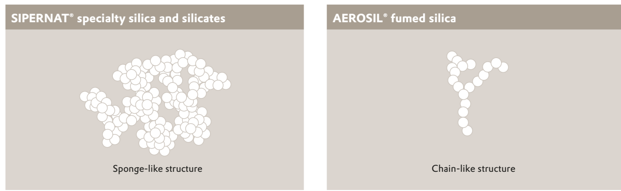
Figure 6 – Specialty silica comparison to fumed silica
