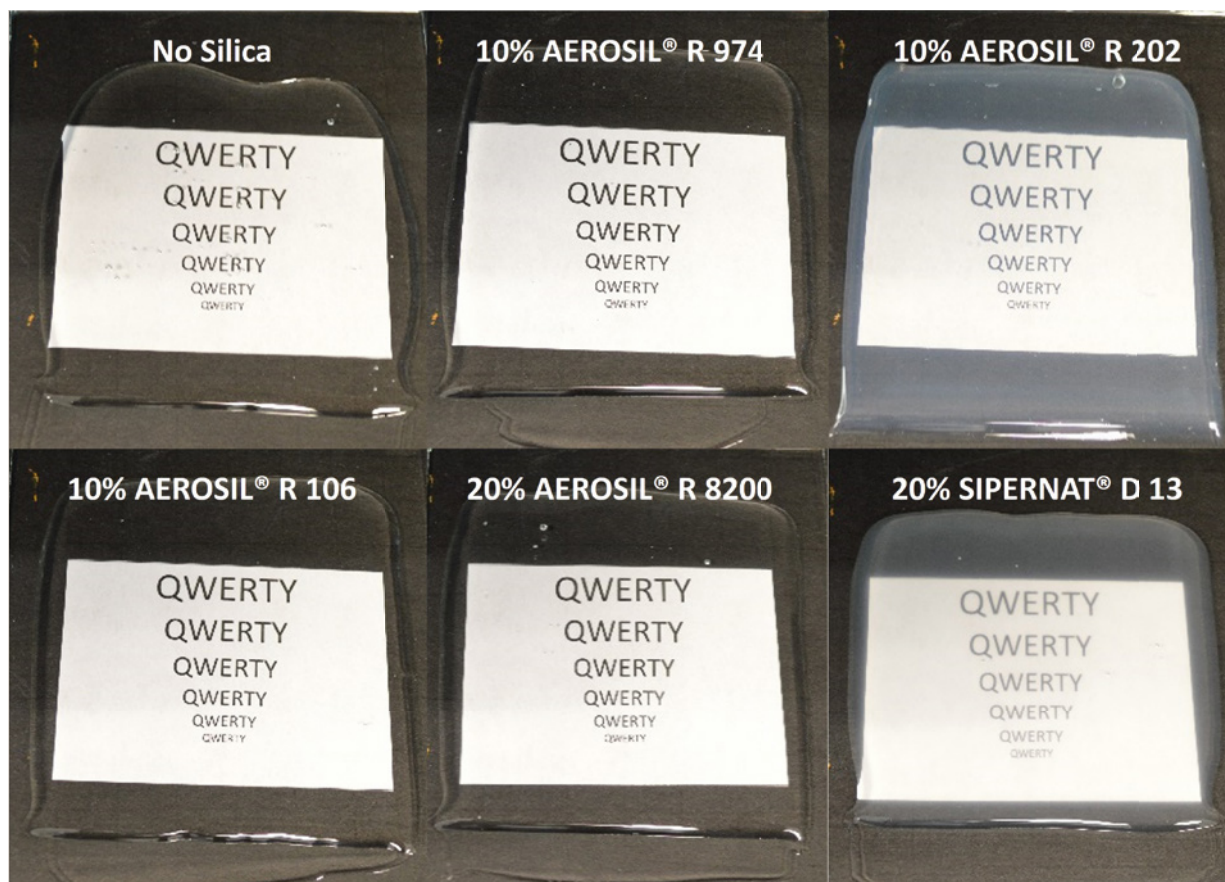
Figure 14 – Silica effect on clarity in STPU Sealant using Polymer ST® 48
