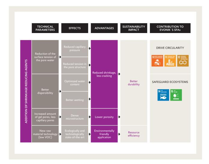
**SITREN® SRA L 201 and 220** are innovative shrinkage-reducing admixtures. These products are designed to significantly minimize both drying and plastic shrinkage in concrete, effectively reducing the risk of cracks, deformation, and debonding thus increasing durability. **SITREN® SRA P 260** is a powder based shrinkage reducing agent based on modified polyethers to prevent cracking of cement based materials.
