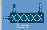
Gases that have higher solubility and smaller molecular size permeate the membrane faster than larger, less soluble gases. The ratio of the transport speeds of two gases is called selectivity.
