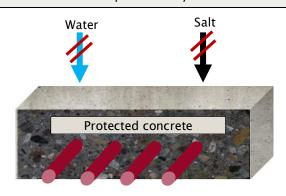
Protectosil® protects the reinforcing steel from corrosion. Chloride ions cannot penetrate the substrate.
