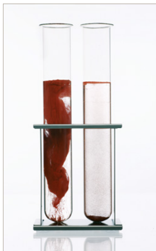
Self-dispersed red iron oxide treated with Dynasylan® 4148 (left) and untreated (right) after 20 s in water
