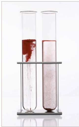
Red iron oxide treated with Dynasylan® 4148 (left) and untreated (right) after 10 s in water
