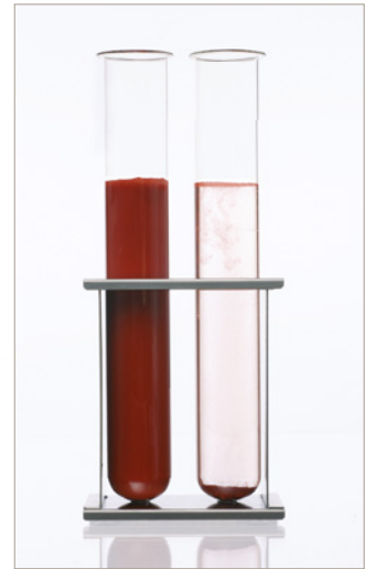
Self-dispersed red iron oxide treated with Dynasylan® 4148 (left) and untreated (right) after 60 s in water
