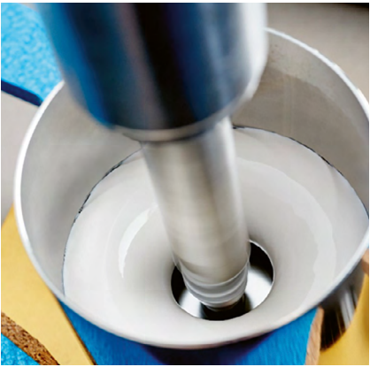
Dissolver dispersion with visible “donut effect”
