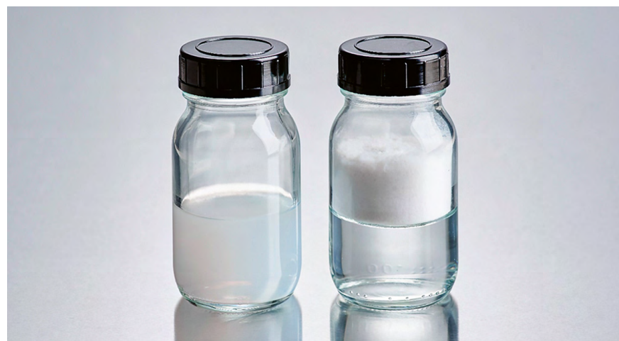
Water with hydrophilic (left) and hydrophobic (right) fumed metal oxide
