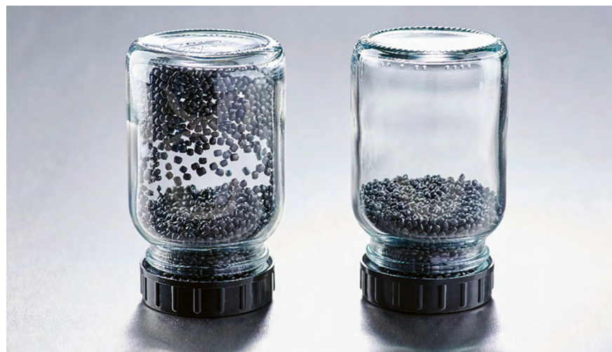
Polypropylenegranulate without (left) and with 0.5 % AEROXIDE® Alu C (right).
