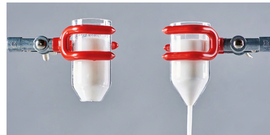
Flow properties of AEROXIDE® TiO 2 P 25 (left) and VP AEROPERL® P 25/20 (right)
