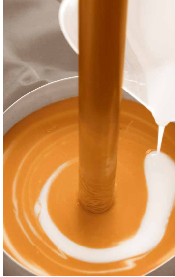
AEROSIL® is used as a rheology modifier in coatings and adhesives formulations, among others. Dispersions are easy to mix with other components.
