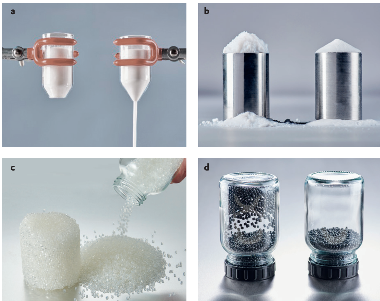
Figure 7a-d Powder flow improvement: a) powder funnel free-flow, b) cone height reduction in powders, c) anti-caking in soft powders, and d) anti-static improvement in non-conductive powders. The powders shown here are only model substances to show the effects as such, and not actual powders for 3D-printing
