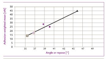
This study demonstrated that mixing conditions need careful attention to ensure optimal dispersion of free-flow agent particles on the powder's surface. Severe mixing conditions should be avoided since they may damage the powder and reduce its particle size, resulting in decreased flowability.
