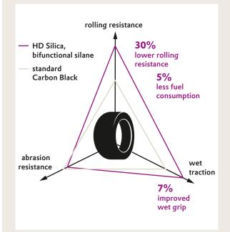
**Figure 2** Silica/Silane system in tire tread
