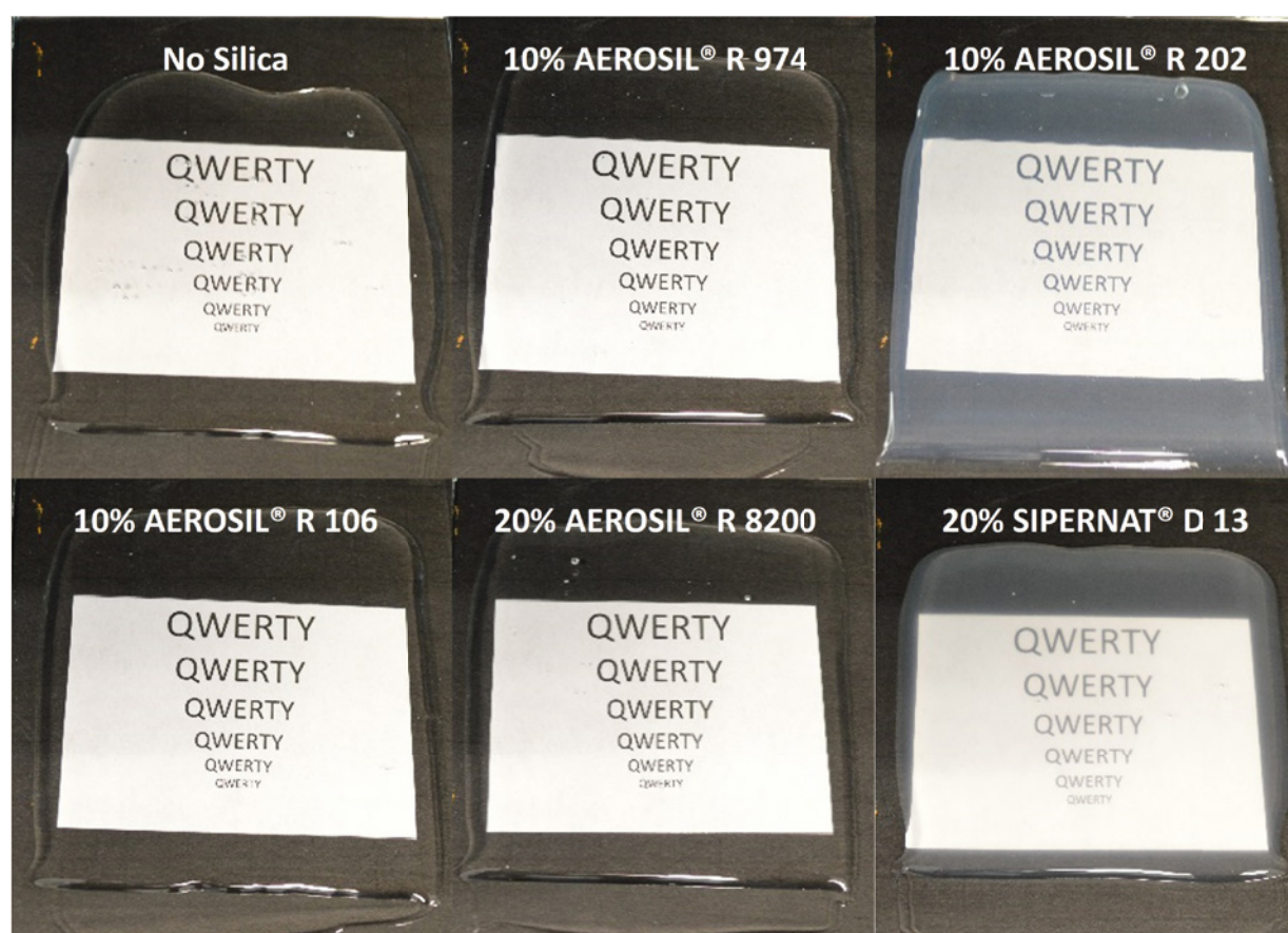
Figure 14 – Silica effect on clarity in STPU Sealant using Polymer ST® 48
