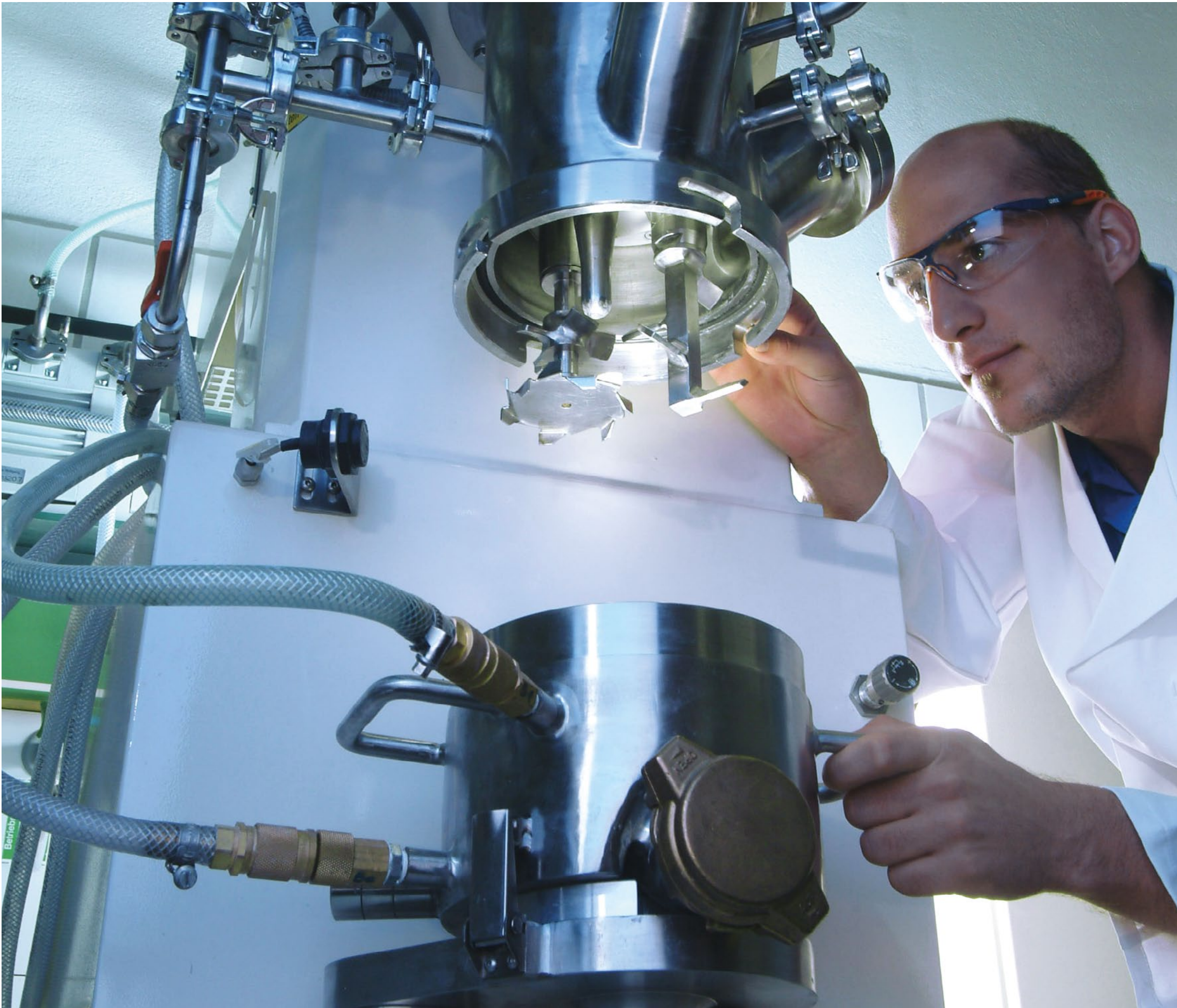
Planetary dissolver for the production of adhesives & sealants (Manufacturer: Hermann Linden, Marienheide/Germany)
