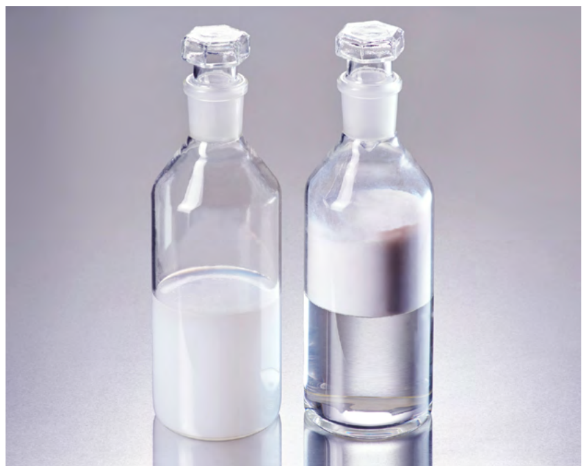
FIGURE 3: Behavior with water for hydrophilic (left) and hydrophobic (right) silica products.
