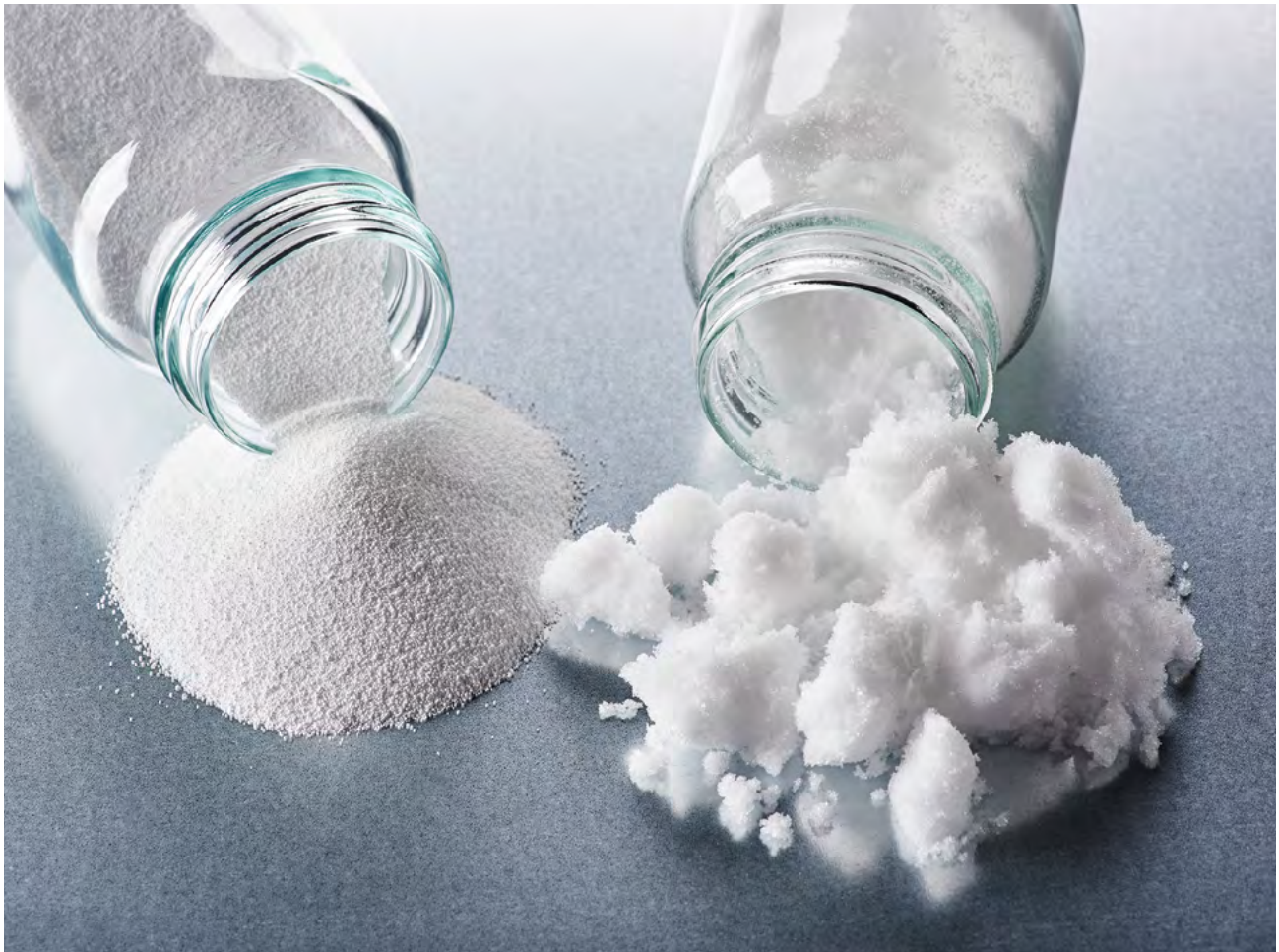
FIGURE 12: Examples of absorbates of the same liquid prepared with different shear forces. Left: low shear mixing Right: high shear mixing
