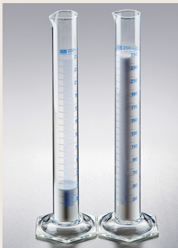
Figure 3 Volume comparison of equal quantities of AEROSIL® 200 Pharma and AEROPERL® 300 Pharma: 8 g of both materials were filled in a graduated cylinder, the one for AEROSIL® 200 Pharma shown on the right and the one for AEROPERL® 300 Pharma on the left.
