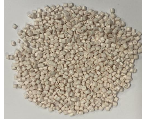
yoghurt cup flakes De-inked with 0.5% TEGO® Cycle WA 111 0.1% TEGOMER® DA 850 compounded
