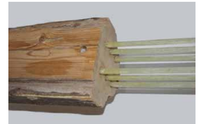
Figure 3: adhesive bonding of glass fiber-reinforced composite rods in a wooden beam for restoration
