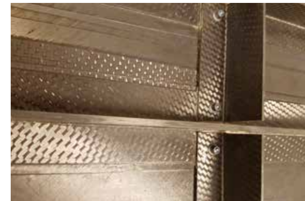
Figure 2: structural adhesive application at the interior of the wing of an Airbus A 380
