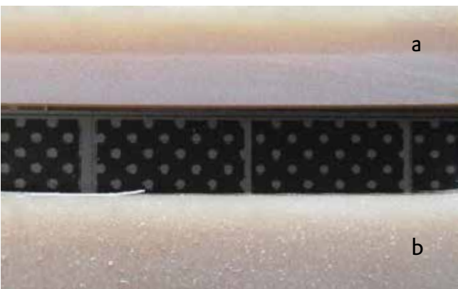
Figure 5: Specimen with \mu -particles only (a) and with micro and nano particles (b). Specimen a shows sedimentation, while NANOPOX® in specimen b prevent a settlement.
