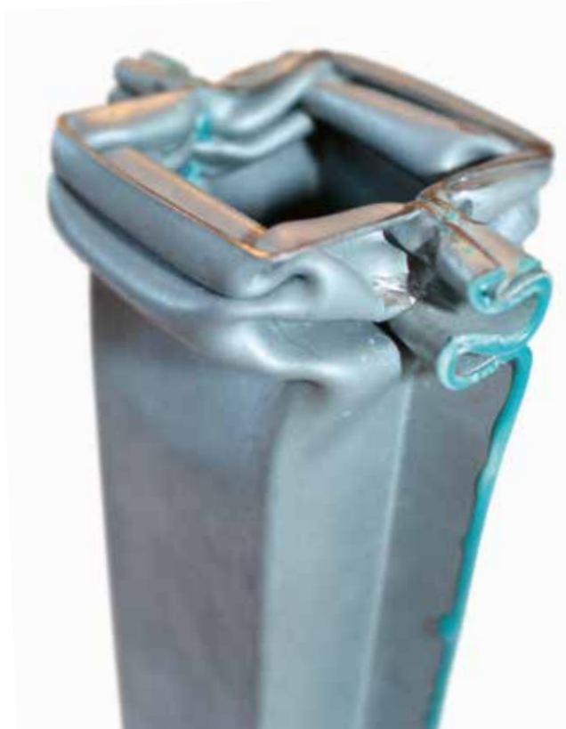
Figure 1: Double hat profile test specimen used to test automotive adhesives regarding crash performance
