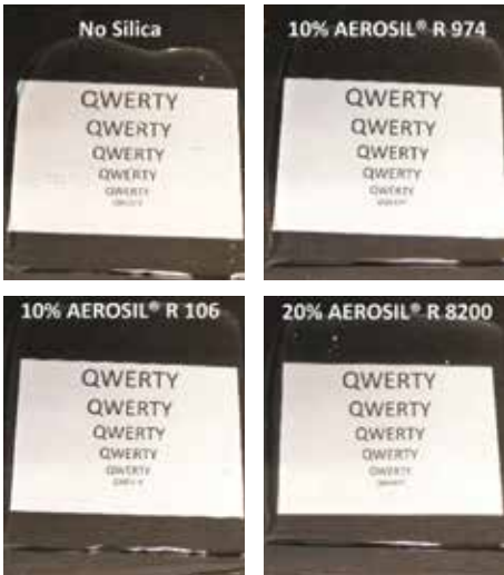
Transparent STPU sealants thickened with each 10 wt.-% of AEROSIL® R 974 or AEROSIL® R 106 resp. 20 wt.-% of AEROSIL® R 8200 in comparison to the reference without AEROSIL® (cf. Formulation 1).
