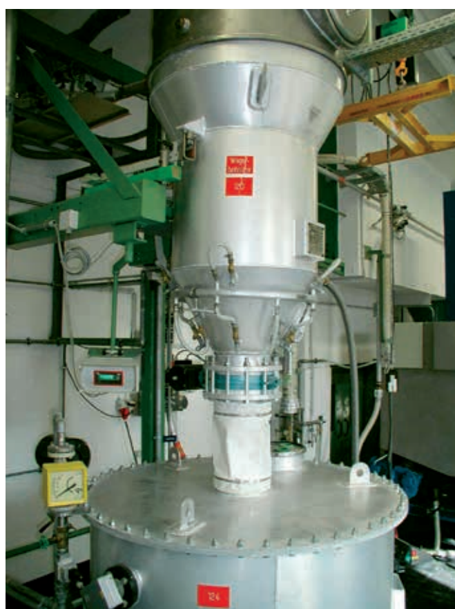
Figure 27 Weighing hopper for the dosage of synthetic silica in batches
