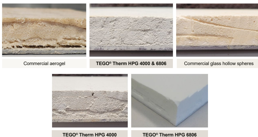
Figure 11. Images of acrylic-based TIC with varying insulation fillers after heat ageing for 10 d @ 140 °C
