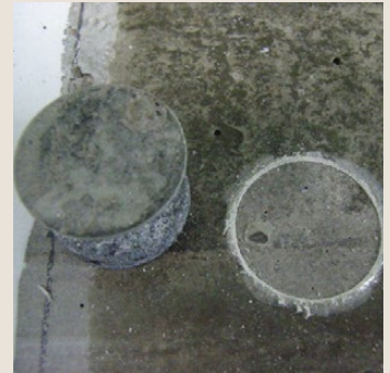
PICTURE 3 145 psi delamination
