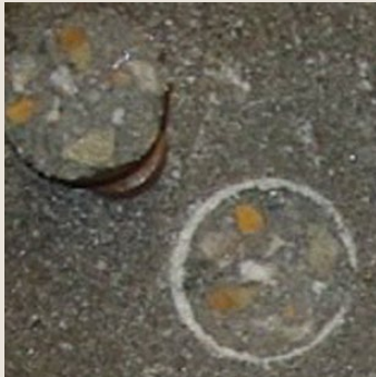
PICTURE 1 1190 psi concrete failure
