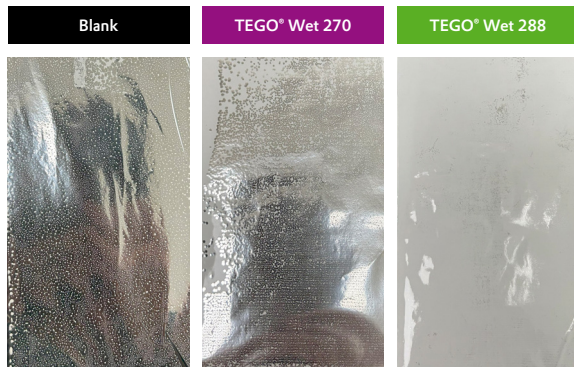
White UV ink applied by hand anilox to metallized BOPP
