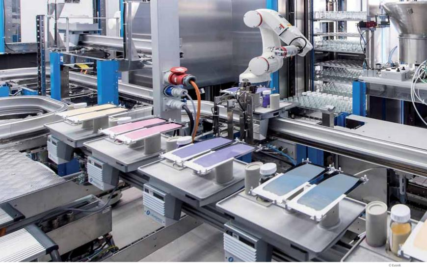
Opening photo: The new, fully automated high-throughput system for testing coating formulations enables to cut down significantly on time spent searching for the optimal formulation.
