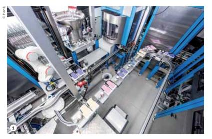
Figure 1: A track system for transporting panels and containers extends through the entire 120-squaremeter HTE system.
