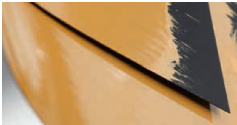
Figure 10: Bad and good flow after brush application
