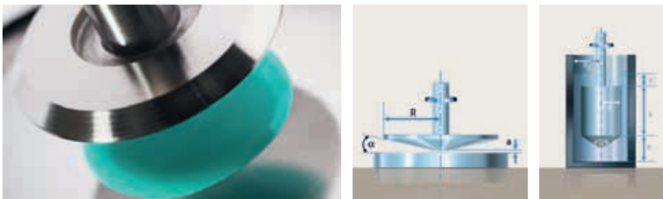
Figure 9: Example for an absolute viscometer and various measuring cells
