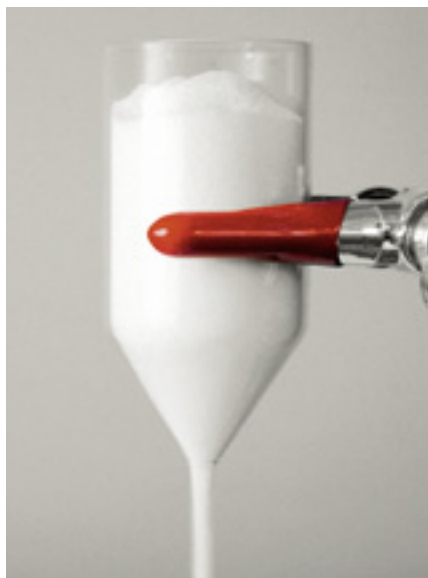
Free flow (left) flow behavior adjusted by use of AEROSIL® R 972 (right) powder coating without AEROSIL®
