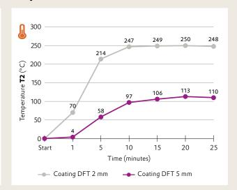
Coatings based on **TEGO® Therm L 300** binder combined with **TEGO® Therm HPG** granules can reach a thermal conductivity ( $\lambda$  value) of less than 40 mW/(m K). Thin coatings with a dry film thickness (DFT) of only a few
