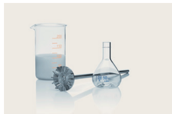
Stirring test: to determine foam behavior in the application of polymer dispersions (e.g. adhesives)
