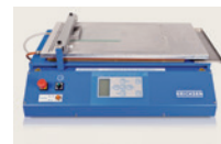
Draw down test: to evaluate wetting and surface defects in film application
