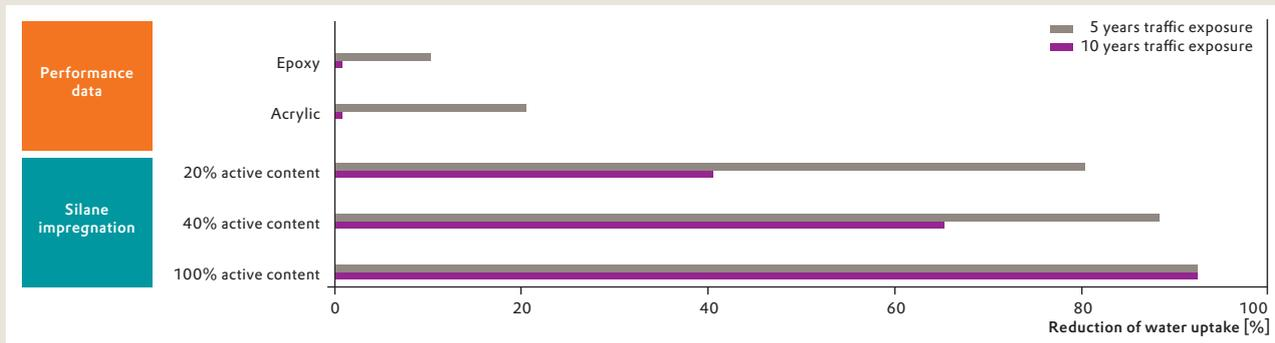
The above diagram shows the reduction in water uptake of a bridge deck's concrete after five and ten years of constant traffic exposure. The higher the active ingredient content of Protectosil® used in the application, the higher the reduction of water uptake and the more durable the protection.
