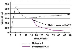
Effectiveness of Protectosil CIT on Chloride Ion Screening After Accelerated Weathering by ASTM G 85 and ASTM D4587
