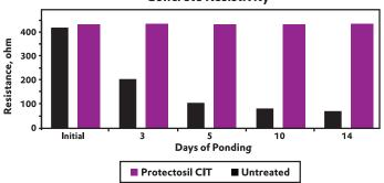
The higher the resistivity or electrical resistance of the concrete, the lower the corrosion current.
