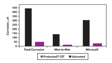
As the chart above shows, the proprietary organo functional chemistry of Protectosil CIT can greatly reduce corrosion currents. This is done chemically by interrupting the electrolytic current and causing a slowdown of the corrosion process.
