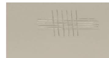
Crosshatch adhesion after 24 hrs curing
