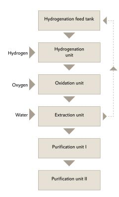
From the hydrogenation feed tank, the working solution containing quinones enters the hydrogenator, where it is hydrogenated in the presence of catalysts to yield hydroquinones. Before the hydrogenated working solution can be fed to the oxidation step, it passes through a filtration unit for complete removal of the catalyst.
