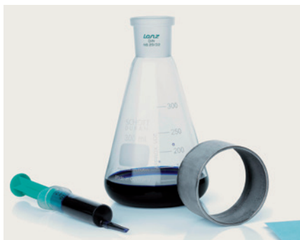
Test ink and Cobb tester for the dye stain test.
