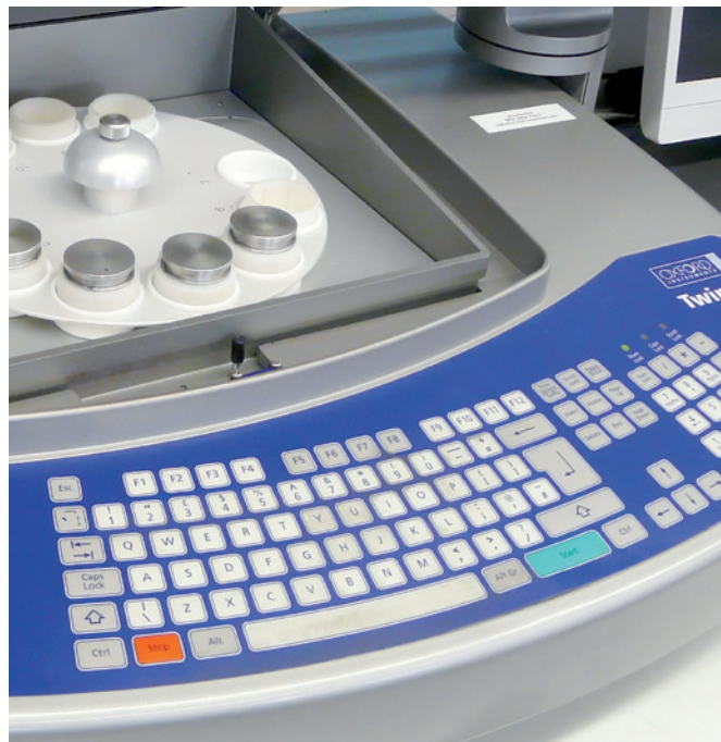
X-ray tester to determine silicone coat weights.
