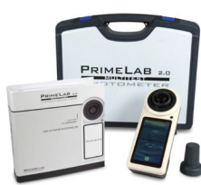
If necessary, turbidity and oxidant concentration are measured with a photospectrometer
