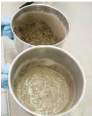
Comparison: mortar without (above) and with (below) SITREN AirVoid® 651
