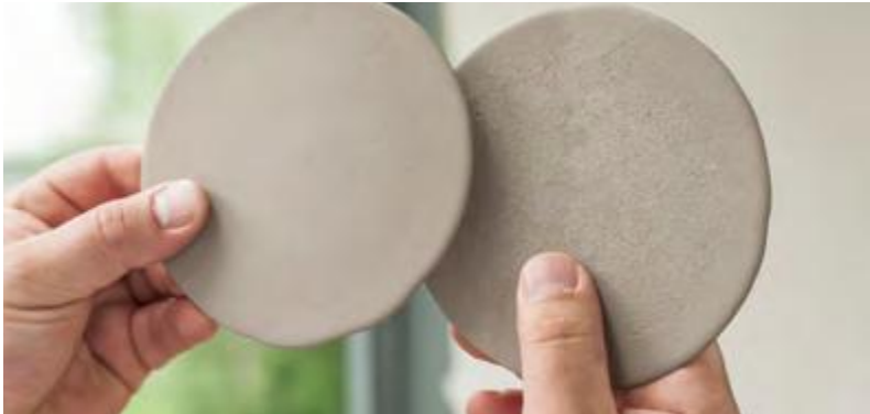
Smooth surfaces, no material build up, high surface hardness with SITREN AirVoid® 370 – Comparison: left with, right without SITREN AirVoid 370®
